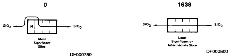
Figure 1-1. Am29203 Arithmetic Shift Path
