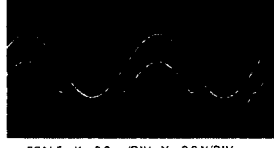
SCALE: X = 0.2 ms/DIV Y = 2.0 V/DIV V_{DD} = V_C = +2.5V, V_{SS} = -2.5V, R_L = 10K\Omega C_L = 15 pF f_{IS} = 1 KHz, V_{IS} = 5V p.p DISTORTION = 3 %
